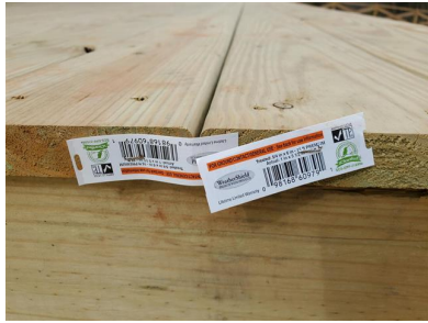
Rear Deck (Pressure Treated/ Ground Contact Wood)
